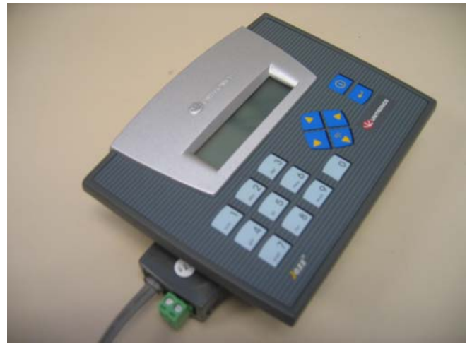
Figure 1.b: The Unitronics Add on Module plugged into the Jazz PLC.
