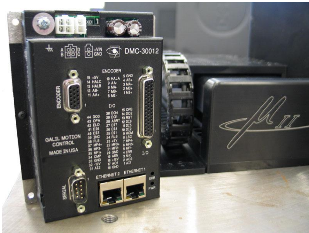
Single Axis Galil DMC-30012 Controller and Drive with \mu II Linear Stage
