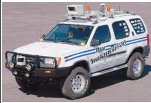
*Team Mojavaton's vehicle, a Nissan Xterra equipped with GPS navigation and other sensors, drives autonomously in the desert based on motion control inputs to the throttle, steering, and braking systems.*
